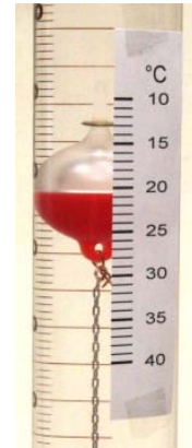
Figure 7. Self-construction of the chain thermometer with calibrated Celsius scale.
