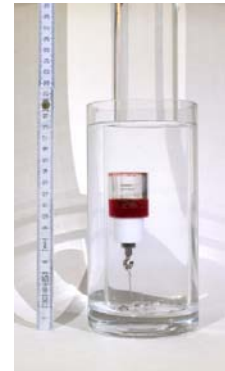
Figure 5. Calibration of the system with an additional little measuring container. Temperature ~ 32 °C.
