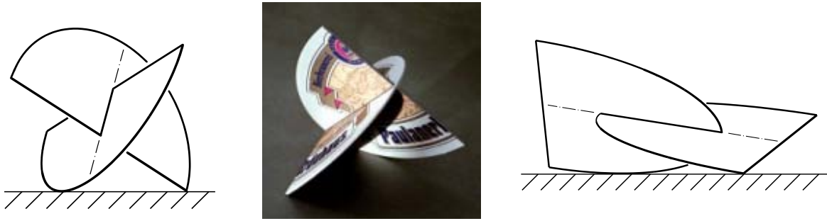
Fig. 18a, b, c: The half-ellipse-roller for negative central distances c , here as the cases a/b = \sqrt{8/7} , a/b = \sqrt{2} , (made of perfectly fitting elliptical beer-mug-stands), a/b = 3 (from the right to the left).
