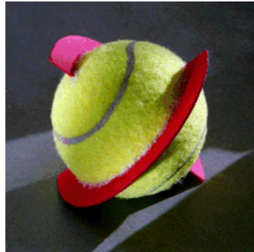
Fig. 20: The tennis ball-two-disc-roller of half-ellipse-discs.
