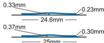
Figure 4. Shapes of original (at the top) and new jumping disc in taut position (not true to scale).
