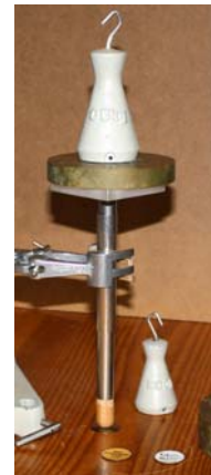
Figure 5. Measurement of force for bending the disc.
