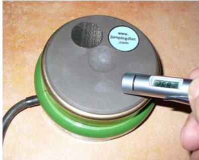
Figure 3. Jumping discs on a small hotplate, with a contactless thermometer on the right.
