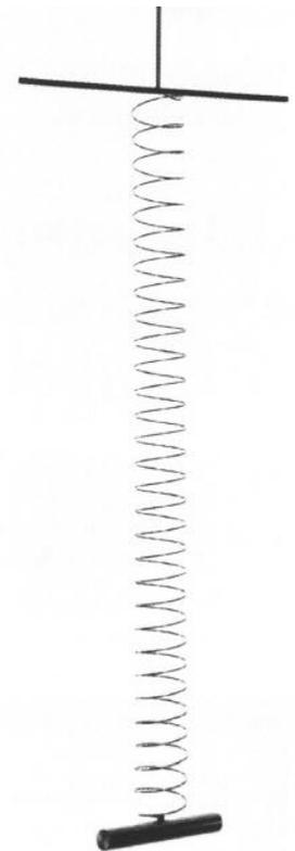
so adjusted that regular switch between vertical oscillations and rotational ones occurs. However the construction of such a rotational pendulum is a bit more complicated because here the pendulum body must be adjusted to the spring with respect to the form (moment of inertia) as well as to the mass. Form and mass of a solid body can hardly be varied independently of each other.
