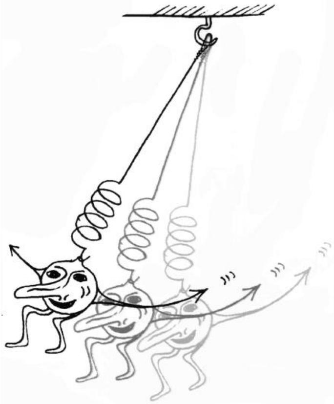
the energy of the oscillations gets dissipated and the pendulum stops moving. What fascinates here both those trained for physics and laymen is the precision with which the two kinds of oscillations switch between each other "at the expense" of each other. However, the unavoidable energy losses due to friction cause the amplitude to get smaller and smaller until the pendulum finish itself at rest.
