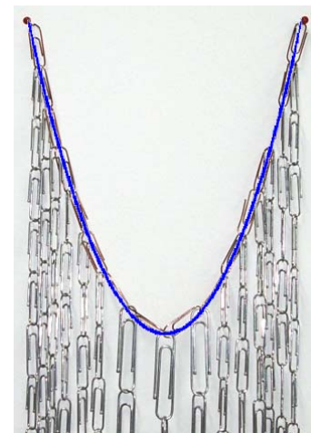
Fig. 5 : Parabola with 16 paper clips and weights. An ideal parabola (blue) is sketched over it. The entire length of the hanging paper clip weights isn't shown here.
