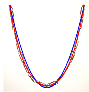
Fig. 4 : Catenary curve with 16 paper clips
