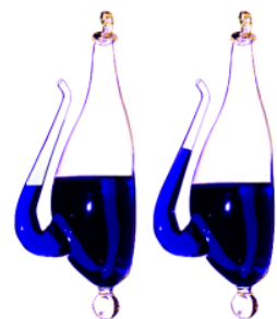
fig.2: High atmospheric pressure leads to a low water level in the spout, low pressure to a high level (at constant temperature).
