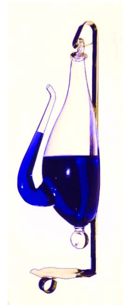
fig.1: Typical weather glass. The round-bodied vessel contains coloured water. Differences in the water level in the beak-shaped spout indicate changes in barometric pressure.
