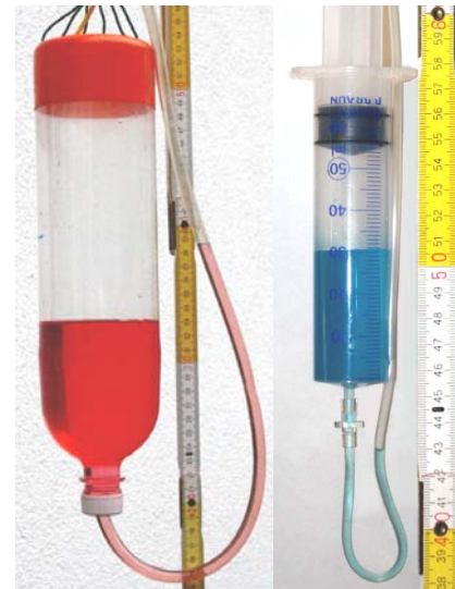
fig.3: construction of a weather glass with a plastic bottle and tube or with a syringe and tube.
