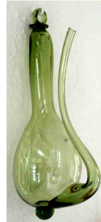
fig.6: Weather glass with an almost cylindrical spout (with permission from [1]).
