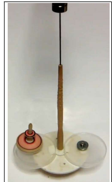
Fig. 4: This self-construction consists of a balance-like arrangement of two disks suspended from a magnet with very low friction. The disks are concave, so that the rotating tops are trapped in them (see video [3]). Here, one top is replaced by an equivalent weight.
