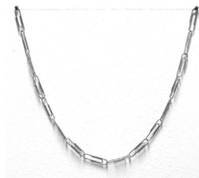
Fig. 1: Catenary curve with 16 paper clips
